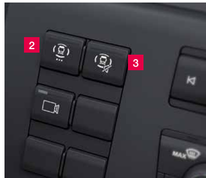
2 Assistance systems button for vehicles without multifunction steering wheel 3 Button for switching off the acoustic signals of the assistance systems
