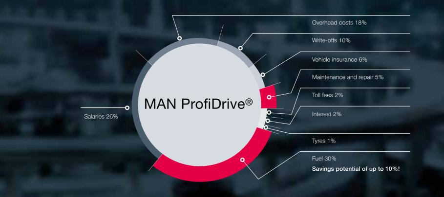
Example of cost distribution for a TGX 18.440 4×2 over a period of four years with an annual mileage of 150,000 km in long-haul transport. The distribution of the TCO may differ depending on the country, type of vehicle and type of operation.
