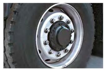
Front axle with hydrostatic wheel hub motors
