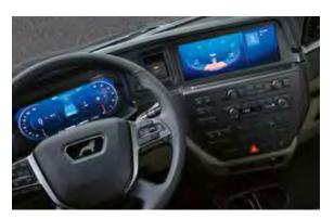
Infotainment system with 12-inch display and control system below the secondary display
