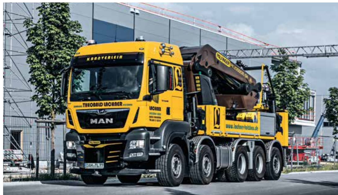
Retrofitted leading axle
