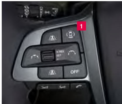
1 Assistance systems button for vehicles with multifunction steering wheel
