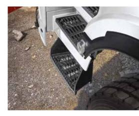
The lowest step, which is prone to damage when driving off-road, is now movable. Its mounting brackets are made from flexible plastic, meaning that they can change shape if they come into contact with the ground and return to their original shape again afterwards. Redesigned air vents: optimal positioning to achieve ideal air distribution and ensure a clear view is achieved again quickly if the windscreen is fogged up or icy.
