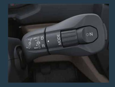
Operation of the gearbox using the right control stalk is a completely new development. Both driving mode and driving program are selected by means of the stalk switch. Controls located in easy reach near the steering wheel and electric parking brake make for certainty in operation.
