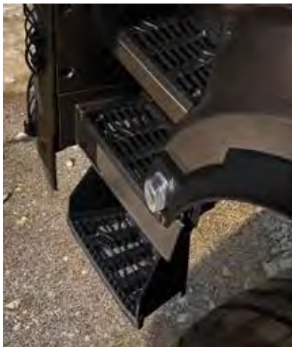
Lowest step fitted with a swing-type function made out of an especially elastic plastic
