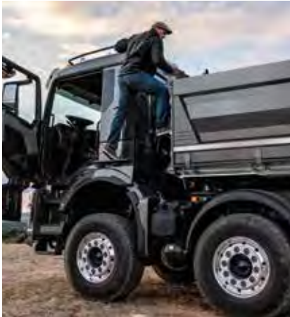
Construction-site rise with support rail on roof
