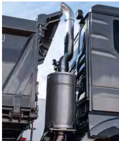
Partially raised exhaust system
