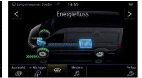
The energy flow display informs the driver about the battery's charge level and the energy flow between the electric motor and high-voltage battery.
