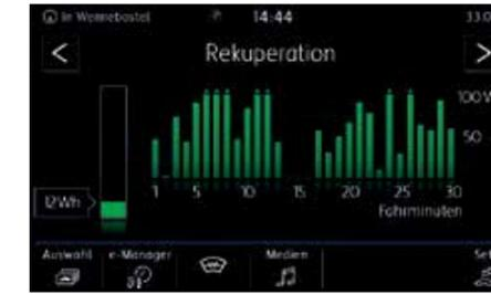
Recuperation is also used to recharge the battery during phases of coasting.
