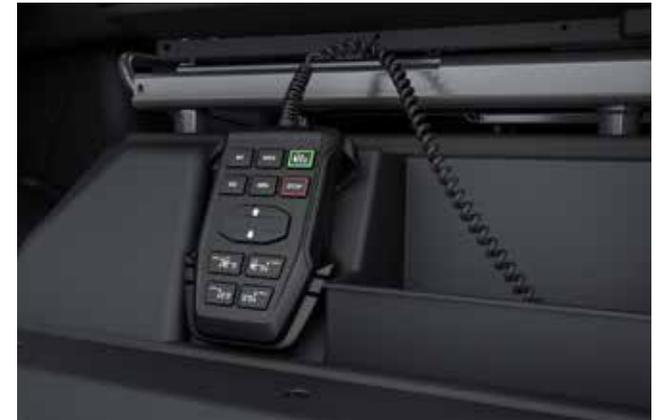
VASC controlling (electronically controlled air suspension)
