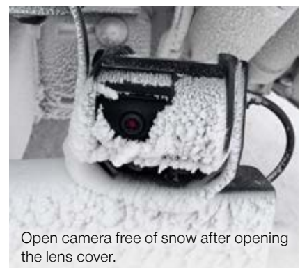
"Eyelid" effect when opening the lens cover.
