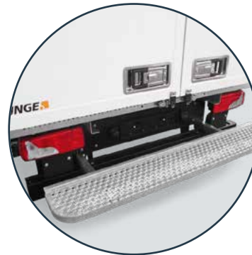
Rear access step Fixed installation spans almost entire vehicle width.
