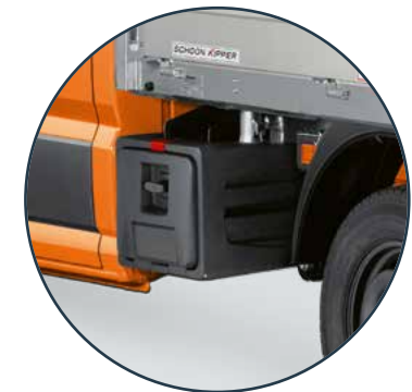
Tool box Mounted under the load area.
