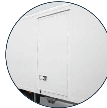
Side door Can be inserted at front right or at back right.
