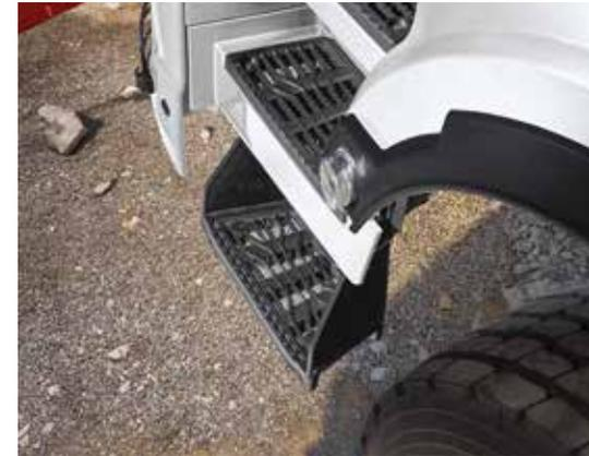
The lowest step, which is prone to damage when driving off-road, is now movable. Its mounting brackets are made from flexible plastic, meaning that they can change shape if they come into contact with the ground and return to their original shape again afterwards.
