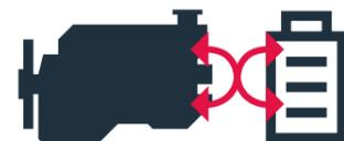
In crossover mode, both drivelines are operated in different operating modes in a two-engine system. Here, one driveline operates in diesel mode, while the electric motor functions as a generator and supplies the electric power for the ship. In the second driveline, the diesel engine is disengaged so that the electric machine receives its energy from the first diesel engine. It operates in motor mode in this case and provides the drive energy.
