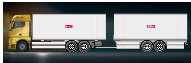
Wheelbase/overhang: 4,800 + 1,350/2,150 mm for solo operation and operation with trailer
