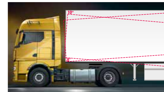
Angle of inclination of fifth-wheel coupling at 150 mm height and tyres 315/70 R 22.5
