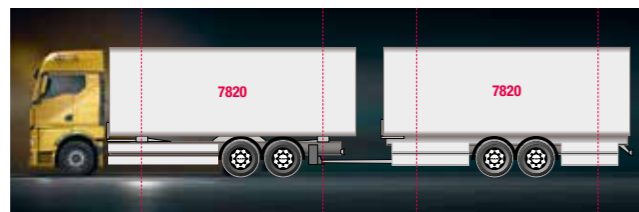
Wheelbase/overhang: 5,100 + 1,350/1,850 mm for permanent operation with trailer
