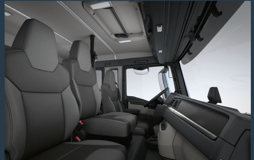
Second passenger seat for the MAN crew cab
